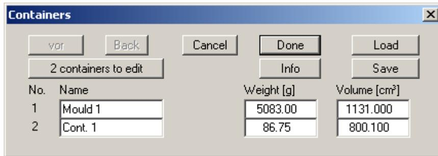
Enter the number of containers to be defined via the "**x containers to edit**" button. The corresponding number of rows for input will then be shown. If more than 8 containers are defined you can navigate through the list using the "**Forw.**" and "**Back**" buttons.
