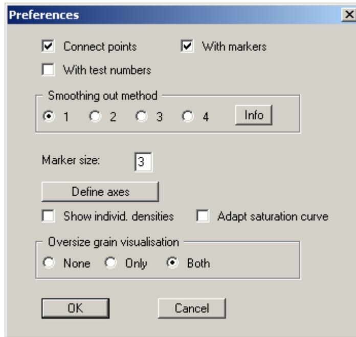
By selecting the "**Connect points**" check box the measured data are connected to form a Proctor curve. This check box will only be deactivated in rare cases, if a Proctor curve is drawn *by hand*, for example. Define how the measured data points appear using the "**With markers**" and "**With test numbers**" check boxes. The marker size is user-defined. If neither of these check boxes are selected the measured data will not be marked.
