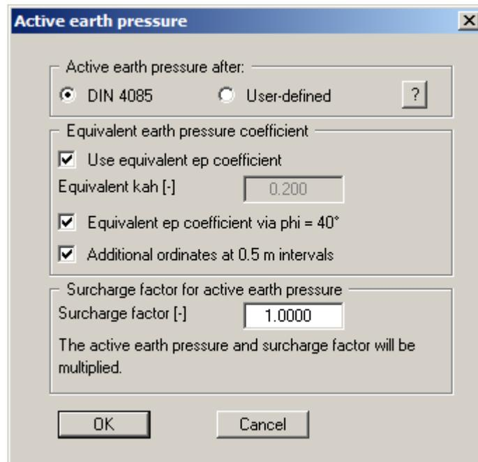
In the upper group box you specify the type of active earth pressure calculation. The method of choice is "**DIN 4085**". The other two methods are only of interest if you wish to analyse an example from older literature sources or check certain results. User-defined earth pressure coefficients can be entered using the menu item "**Editor 1/User-defined earth pressure coefficients**" (see Section 8.2.13).
