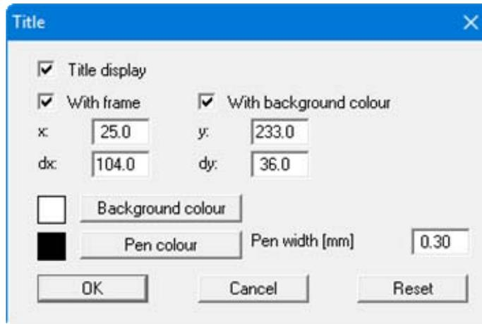
The position of the element on the output sheet and its size can be defined or edited by means of the variables "x" and "y", "dx" and "dy". The element can be provided with a frame and a background colour to suit your personal requirements. If the element needs to be returned to its original condition, this can be done using the "Reset" button. Alternatively, you can alter the size and shape of the element using the mouse (see menu item "Output preferences/Move objects", Section 5.4.21).
