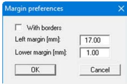
By deactivating the "**With borders**" check box and with an appropriate choice of left and lower margins, it is generally possible to create a non-reduced printer output. It is necessary to also adapt the page height and width (see Section 5.4.1).
