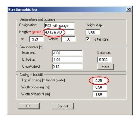
The height of the casing *relative to ground level* is entered in the "Casing + backfill" input group box. If the pipe protrudes from the ground the height difference must be entered as a negative value (also see the example in Section 5.3.4).
