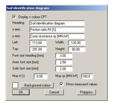
The soil identification diagram was developed from test series' in which the friction ratio was drawn against the cone resistance for a variety of soil types. This results in different polygons used to identify the soil types. They can be adapted for typical local evaluations using the "**Polygons**" button and saved in an "**.idx**" file. A soil type can be determined using only the CPT data by colour evaluating via the defined polygons.
