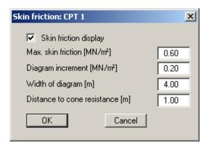
With "**Distance to cone resistance**" you can control the distance of the skin friction diagram to the cone resistance diagram. Using the program defaults it will be displayed with a spacing of one metre (= 1 cm at a scale in x-direction of 1:100) to the left of the cone resistance diagram.
