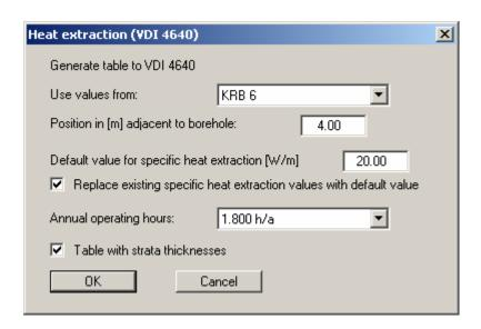
In the "Ex\_Geothermal energy.bop" example file the ground source heat table is shown adjacent to hand percussion bore KRB 6. If a new VDI table is created and a number of boreholes are available, the borehole with the depth data for adoption in the table can be selected using the drop-down menu in the dialog box. Define the position of the table as the distance from the right edge of the selected borehole. The value of x in the base data is adjusted accordingly.
