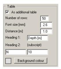
To achieve visualisation with a table row corresponding to a penetration depth of 10 cm (same graphical end depth for both the diagram and the table), define a font size of *1.3 mm* for an overall image scale for the y-direction of *1:50*. The font size in the example file should therefore be 2.6 mm for a scale of 1:25.
