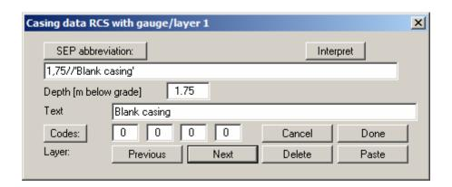
When entering the layers for the casing the difference to ground level must be either subtracted from or added to the depth of the pipe, as appropriate. If a 2 m long blank casing protruding 0.25 m above the ground is used, the length of pipe in the ground is entered as a depth of 1.75 m for casing layer 1.
