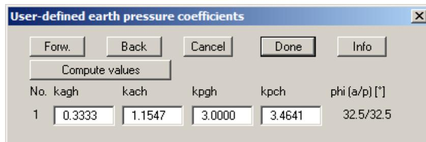
If the "Compute values" button is pressed the earth pressure coefficients can be calculated by the program in accordance with the required standard and slope angle.
