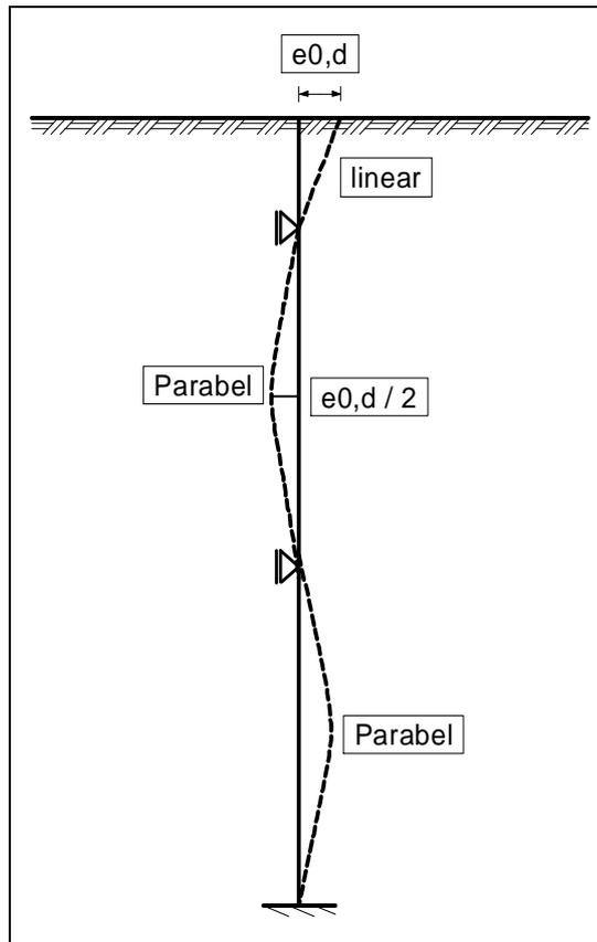
Figure 11 Pile with two displacement boundary conditions
