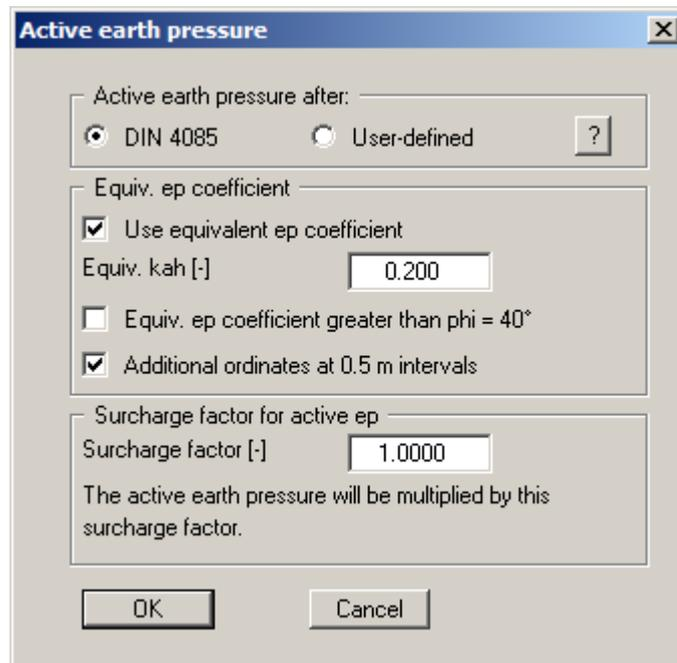
In the upper group box you specify the type of active earth pressure calculation. The method of choice is "**DIN 4085**". The other two methods are only of interest if you wish to analyse an example from older literature sources or check certain results. User-defined earth pressure coefficients can be entered using the menu item "**Editor 1/User-defined earth pressure coefficients**" (see Section 7.2.10).
