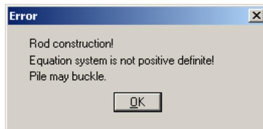
The normal force given in the data files thus corresponds to the buckling force determined after Euler.
