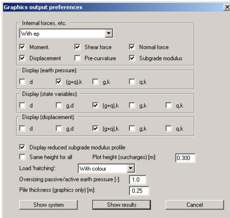
If a system has been analysed using 2<sup>nd</sup> order theory with buckling analysis to DIN EN 1993-1-1 activated, either the "**Displacement**" or the "**Pre-curvature**" can be selected for display in the result graphics in the dialog box shown above. Any adopted pre-curvature will always be given in the output table.
