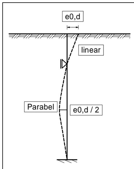
Figure 10 Pile with a displacement boundary condition ( $w_x = 0$ )
