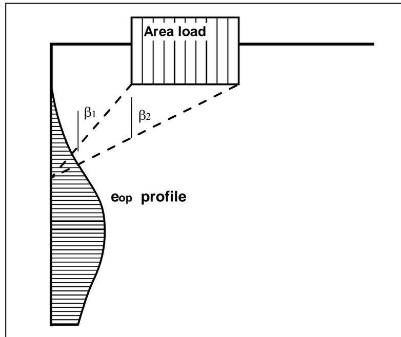
Figure 6 At-rest earth pressure from area loads
