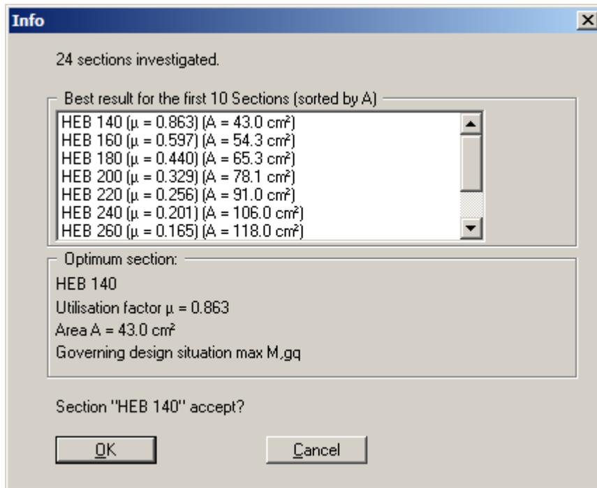
The analysis and design of the pile are complete. The input and results are first displayed in message boxes, which you move through by clicking "OK". Because a different section to the originally selected HEB 300 was designed, the analysis should be repeated using the new HEB 140 section. Adopt the pile width of the newly selected pile by pressing the "Adopt" button and repeat the analysis and subsequent design of the HEB 140.
