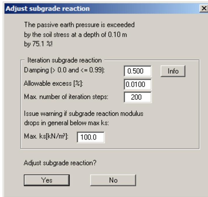
The program has determined that the passive earth pressure is smaller than the resulting soil pressure from the elastic analysis, which is not permitted. An iteration process must be carried out. In the dialog box shown above, you can enter the iteration conditions. The *default values* have proved themselves in practice and will generally not need to be altered.
