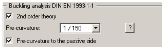
The size and direction of the pre-curvature can be specified. Whether a pre-curvature towards the passive side or the active side provides the more unfavourable design values is system-dependent: the following message will therefore be displayed once analysis begins:
