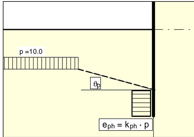
Figure 8 Bounded surcharge (passive side)
