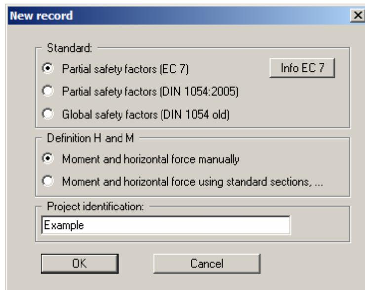
In the upper group box of this dialog box select the safety factor concept for analysing your new system. Specify how to define the moment and the horizontal force in the middle drop-down list box (also see the "**Edit/System parameters**" menu item, Section 6.2.2).
