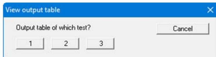
The "1", "2" etc. buttons represent the tests entered. The most important test data can be viewed for every test. If more than 35 measurements are available for the selected test the number must be reduced for the output sheet.
